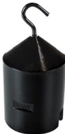
Figure 1: A 1 kg cast iron lab weight. Its gravitational potential energy will be the sole power source for the vehicle.
