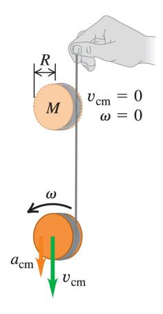
A yo-yo of total mass M is formed from two uniform solid disks of radius Rconnected by a massless axle of radius  $R_0$ . The yo-yo unrolls on a string wrapped around the axle starting from rest through a vertical height h.
